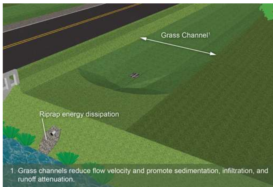
Figure 10.6.2-1 - Typical grass channel configuration
