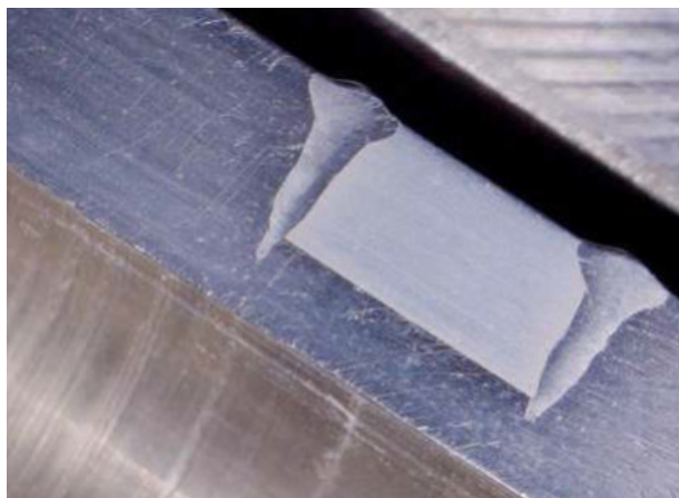
An electron beam cross-sectioned weld spike
