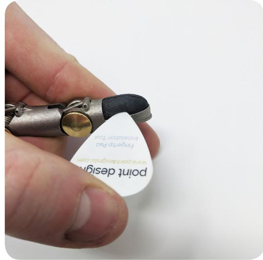
**2.** With the pad partially pried up, use your fingers to grab the pad and pull it the rest of the way out.
