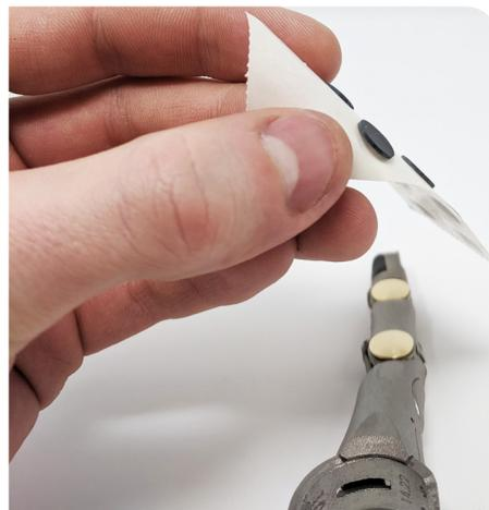
**3.** Center over the joint, then press on to the Chicago Bolt and hold pressure for at least 10-20 seconds. Clamping the pad down for 72hrs will yield optimal results, but is not necessary.
