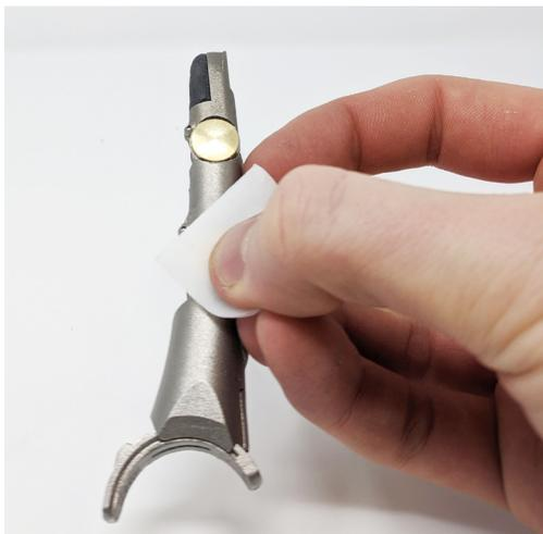
**2.** Remove the Lateral Grip Pad from the backing
