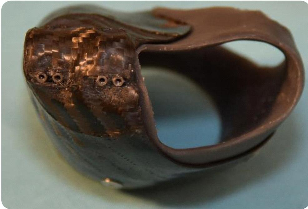
17. After curing is complete and the model has cool, clean up the prepreg and remove the lamination spacers.
