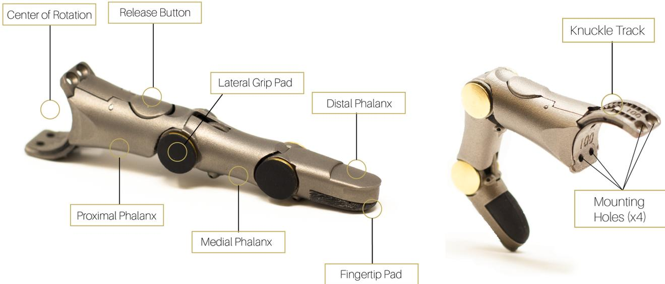
The **Point Digit** comes assembled as one unit. The **Point Digit** is comprised of a curved knuckle track, proximal phalanx, medial phalanx, distal phalanx, a release button, fingertip pads, lateral grip pads and several other internal parts. The curved knuckle track has 4 mounting holes.
