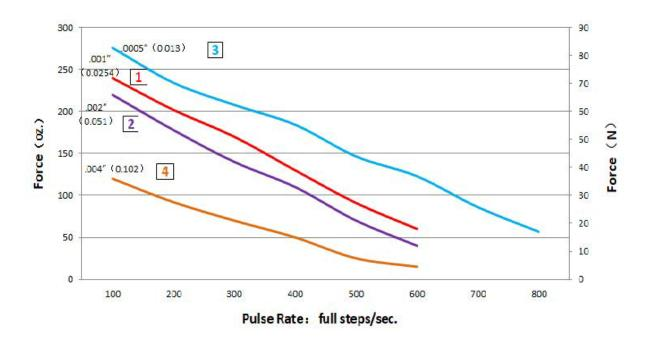
25% Duty cycle is obtained by a special winding or by running a standard motor at double the rated current. With L/R drives peak force and speeds are reduced, using a unipolar drive will yield a further 30% force reduction.
