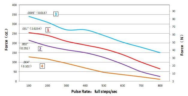
25% Duty cycle is obtained by a special winding or by running a standard motor at double the rated current.
