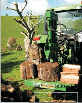
For larger tractors the Agriquip three point linkage mounted Hydrasplitter puts hydraulic power into use with unrivaled force. These splitters feature a simple, easy to use control valve with a convenient detent to return the ram quickly - ready for the next operation. The VTL can be used from a position sitting on the ground, to a point anywhere in the range of the tractors draft arm lit range, to suit any operator.
