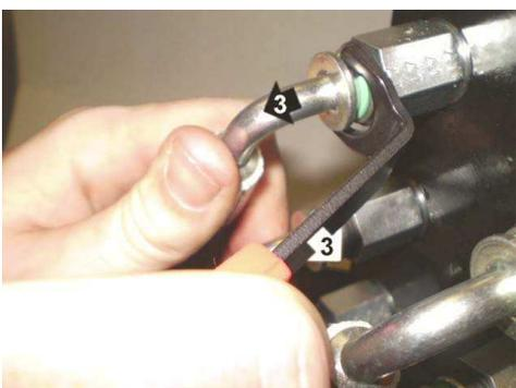
(3) Lever removal tool outwards and decompress the fitting (*rearwards*).
