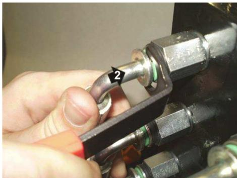
(1) Locate removal tool behind collar of hose end fitting. (2) Compress fitting (*forwards*).
