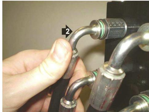
(1) Locate hose end in receiver fitting. (2) Press fit into position (*pull on fitting to check*).
