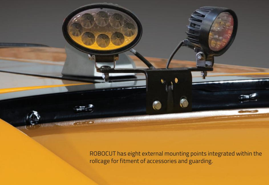
ROBOCUT has eight external mounting points integrated within the rollcage for fitment of accessories and guarding.
