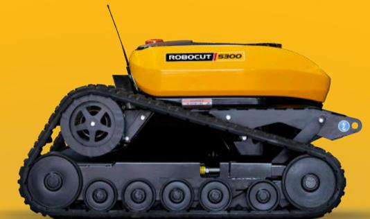
The S300 features a specially designed 1.1m bi-directional rotary mulching deck for cutting in either direction. Ideal for producing a quality cut and attractive finish in fine turf applications such as parks and gardens, whilst tough enough to be used for extensive mowing of heavy grass.
