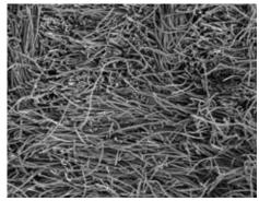
Extended-life needle felt in comparison to standard needle felt - Finer fibers - Greater porosity
