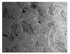
Surface of a DURAGAF filter bag - No fiber release - Full flow through surface channels
