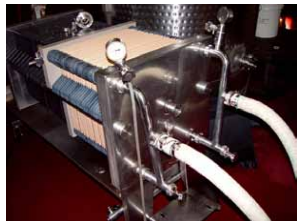
Figure 2—Typical Filter Press or Sheet Filter
