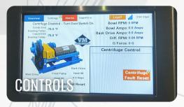
Vision View allows you fully functioning remote access to your centrifuge and ancillary equipment. Vision View allows you to monitor and troubleshoot remotely via mobile access or computer.
