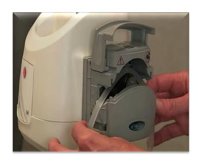
NOTE: position tubing so fluid will run from blunt portion of arrow (bag) to pointed end of arrow (patient); arrow is located on various points of pump depending on model.
