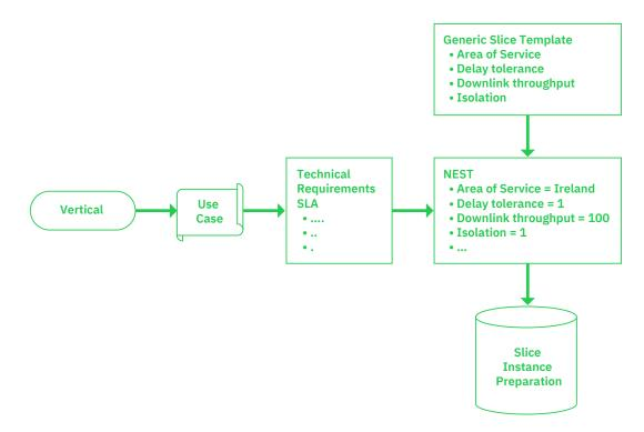
Figure 3: Path from Use Case to Slice Instance Preparation
