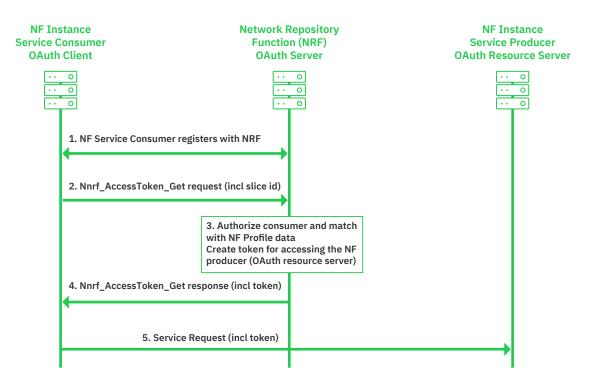
Figure 4: Network Function Consumer Obtaining Access Token from NRF for Service Usage
