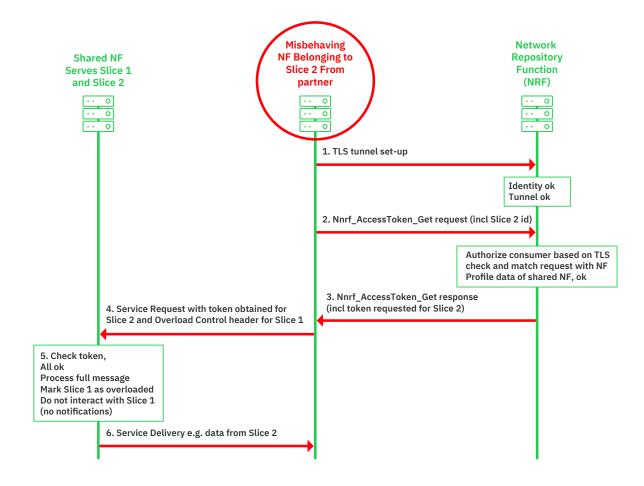
Figure 13: Potential DoS Attack Against Slice Network Functions
