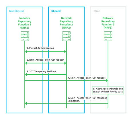
Figure 5: Slice Specific NRF - Forwarding of Requests from TS 29.510 [7]
