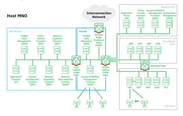
Figure 16: Example Security Zoning in Sliced Network
