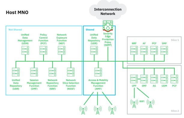
Figure 2: Example Slicing in the Core Network
