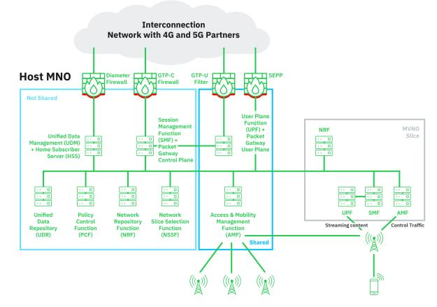
Figure 9: Legacy Roaming and Interface Protection
