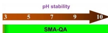
pH stability of SMA-QA, adapted from [2]. Stabilizing pH range shown in green.
