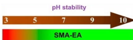
pH stability of SMA-EA, adapted from [2]. Stabilizing pH range shown in green
