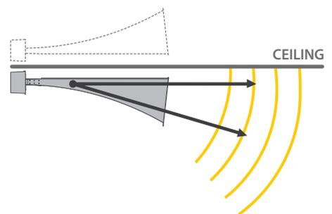
that the introduced S4T solution allowed clean transmission of clear and understandable messages to the tunnel users. Narrow angles of radiation and the ability to produce high sound pressure levels without distorting the audio signal makes ABT-TNL100 an ideal solution designed for noisy environments of road tunnels.
