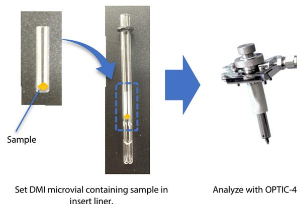
Fig. 2 Sampling Procedure for Pyrolytic Analysis Using OPTIC-4
