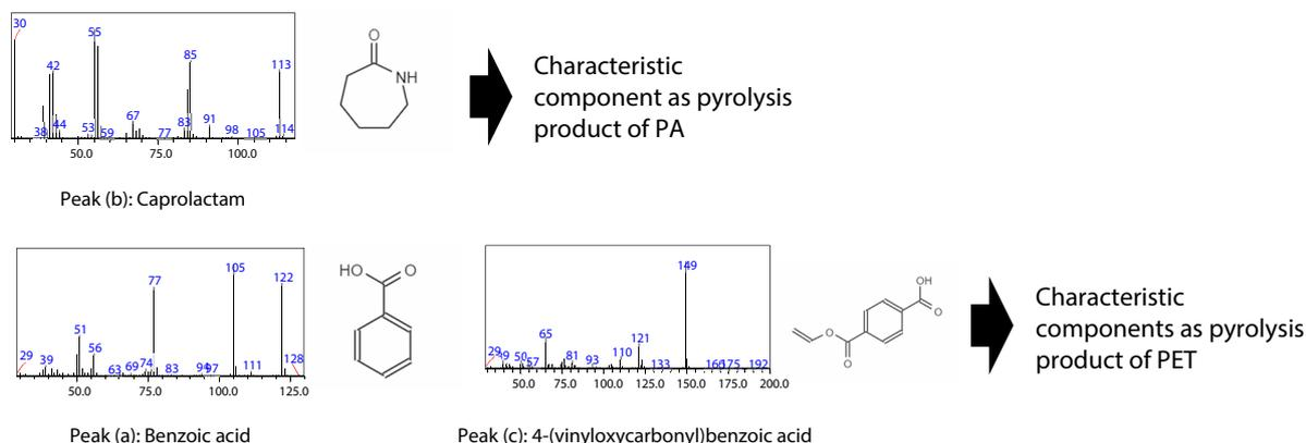
Fig. 4 Mass Spectra of Peaks (a) to (c) and Identified Compounds
