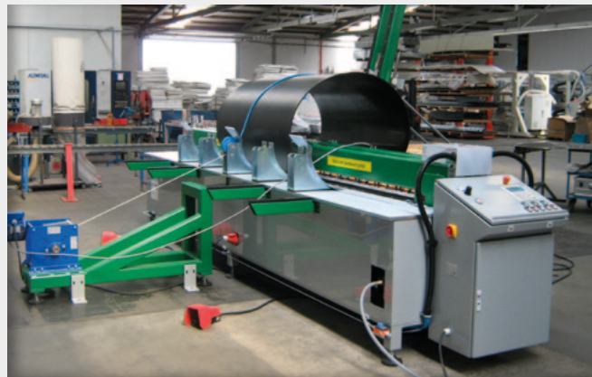
Sheet rolling unit RZ-V 1.0 for sheet thicknesses between 5 - 25 mm and diameters between 500 - 3,000 mm
