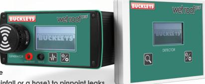
The kit comprises two main elements; a generator unit and a detector unit. The generator unit creates an electrical field across the roof surface via a 'boundary wire' which is positioned around the perimeter of the test area and connected to the positive terminal on the generator unit. The negative terminal is connected to a suitable earth on the building's structure.
