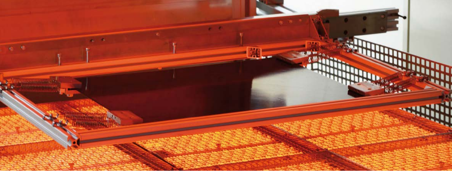
Homogeneous heating of an organo sheet Source: Fraunhofer IPT
