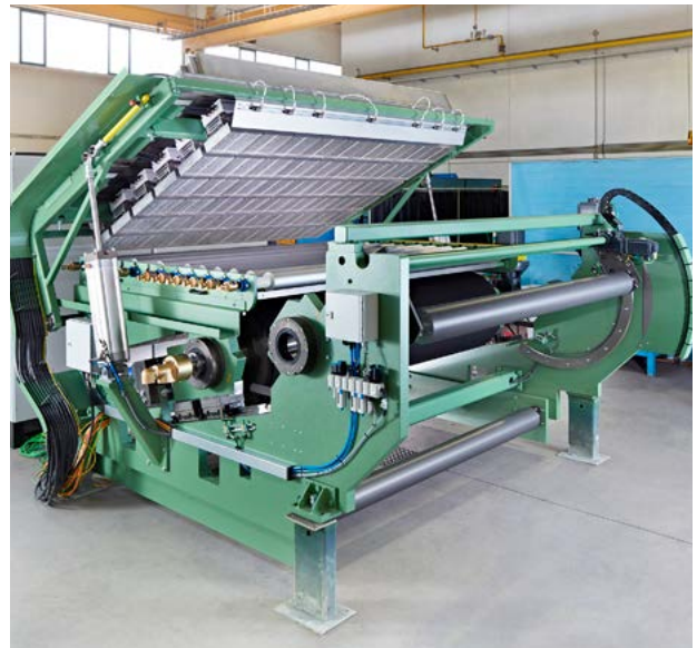
KRELUS infrared preheating for embossing machines Source: Kampf LSF GmbH, Laussig, Germany
