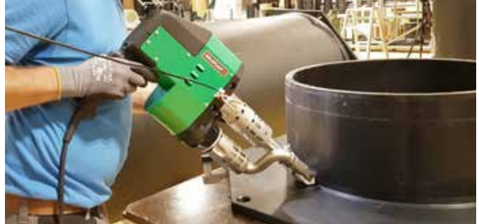
The powerful WELDPLAST S4 in use.
