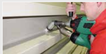
The 45° angled adapter for the WELDPLAST S2 facilitates welding in difficult positions. (accessory)
