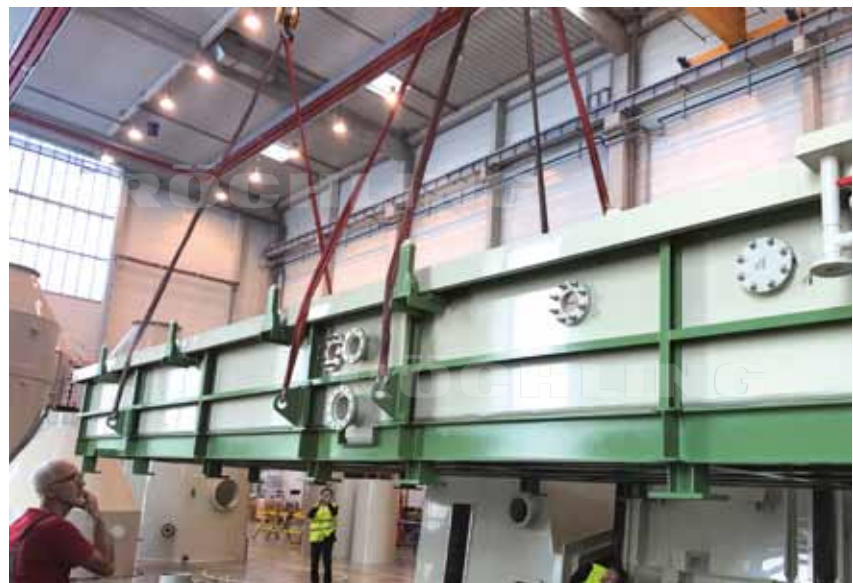
Polystone® P homopolymer grey extra heat stabilized for a steel-pickling plant
