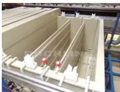
Polystone® P homopolymer grey Process tanks in a plastic electroplating
