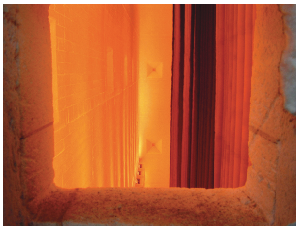
Figure 5. Typical side fired flat flame burner installation in an ethylene cracking furnace.
