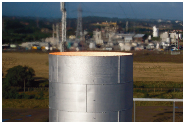
Figure 8. Refinery ground flare installed to limit light and noise pollution during routine flaring.
