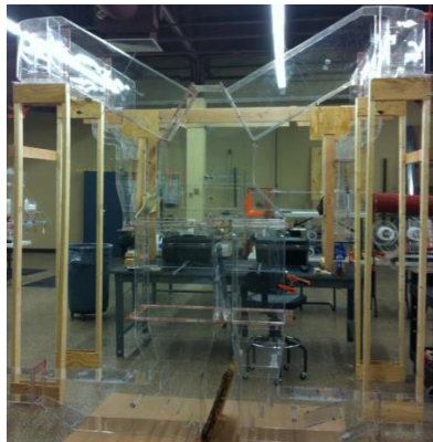
Figure 6: Free-Jet Physical Flow Simulation
