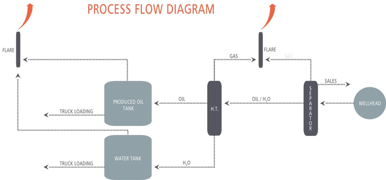
**Figure 2:** Wellpad Process Flow Diagram
