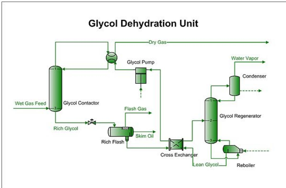
**Figure 3:** Glycol Dehydration Unit Flow Chart
