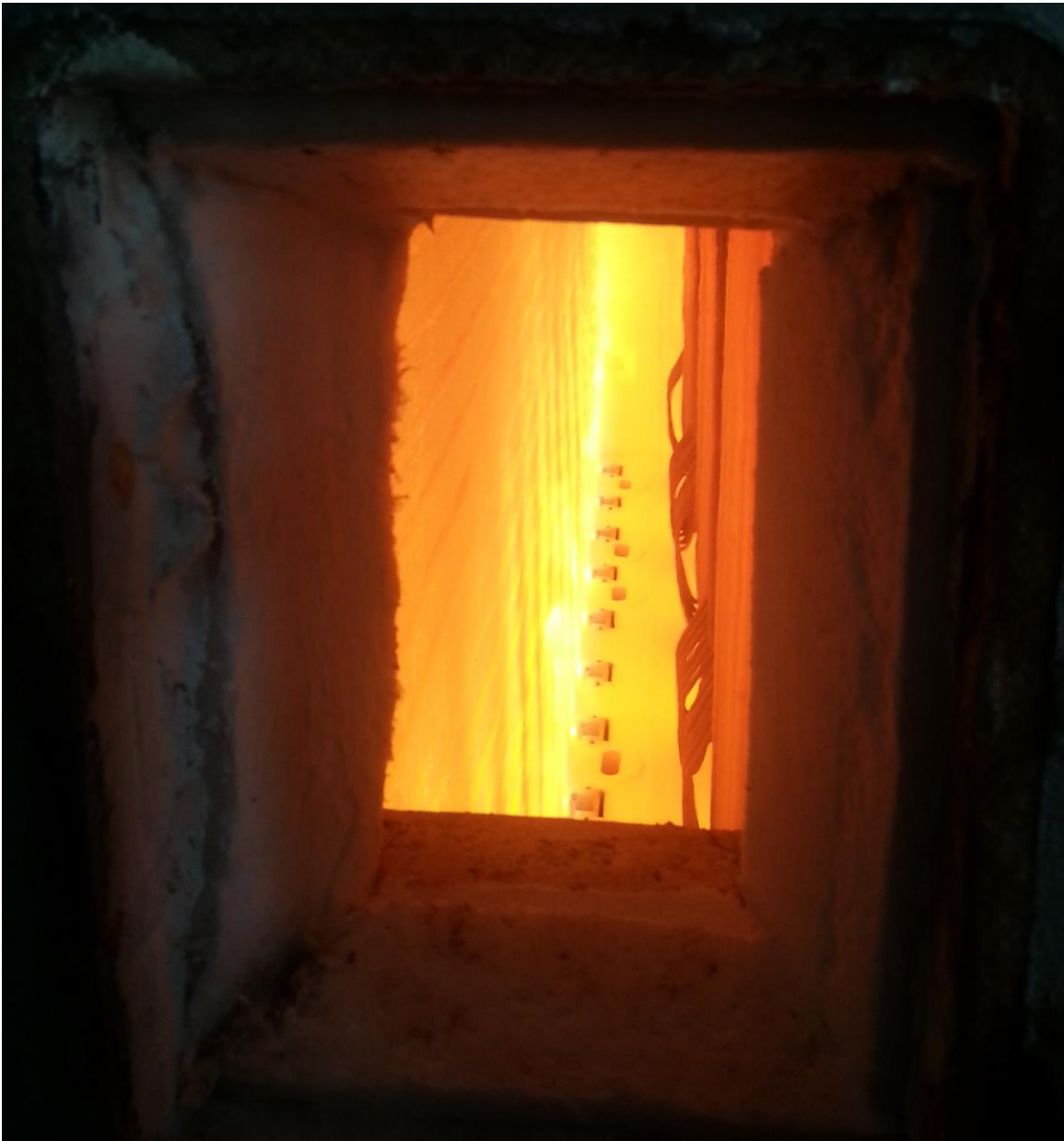
Figure 1: The burner is designed so the gas stays next to the wall. Therefore, when the furnace currents pull the air toward the tubes, the gas and flame remain next to the wall with no flame rollover.
