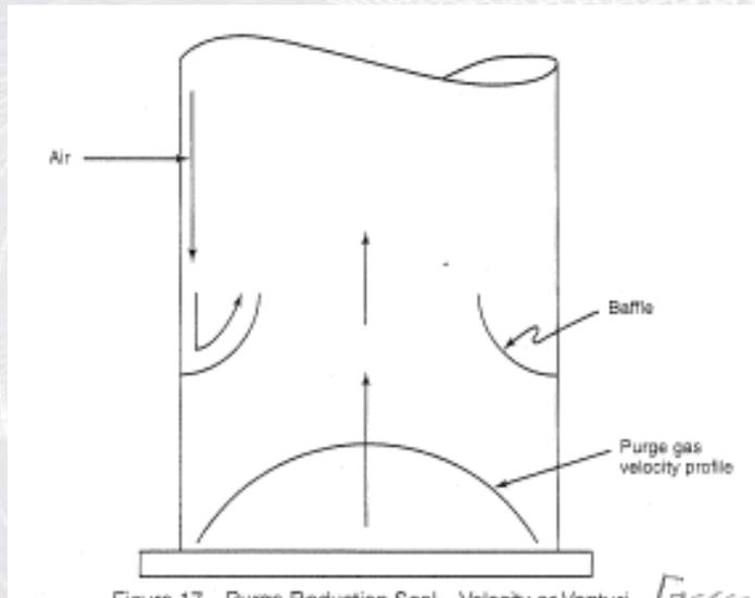
Figure 17—Purge Reduction Case—Velocity of Venturi
