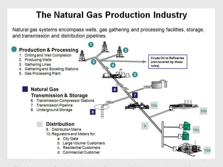
The Natural Gas Production Process Diagram adapted from the American Gas Association and the EPA Natural Gas STAR Program
