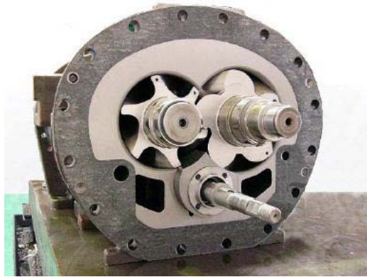
Figure 10. Typical Flooded Screw Compressor Internal View
