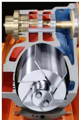
Figure 12. Typical Sliding Vane Compressor Internal View
