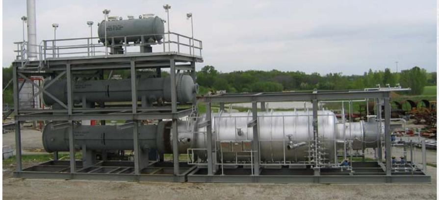
Modularized SRU Reaction Furnace
