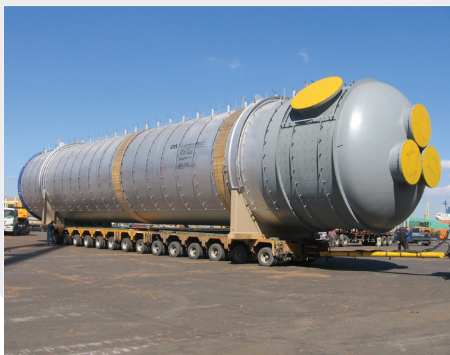
World's largest SRU tail gas incinerator — one of nine similar incineration systems supplied by Zeeco
