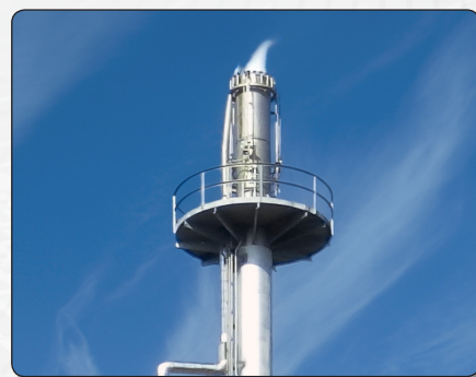
Improper application of steam
