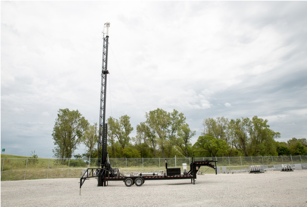
Figure 2. 60 ft trailer-mounted guy-wire supported temporary flaring system, typical of system supplied by Zeeco for this rental application at an LNG facility.
