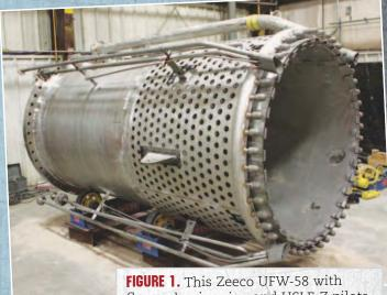
flame shaping ring and HSLF-Z pilots was produced for one of the world's largest LNG producers through the Zeeco Rapid Response Team.
