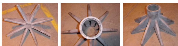
Figure 3. Zeeco's pressure-assisted flare tip casting.
