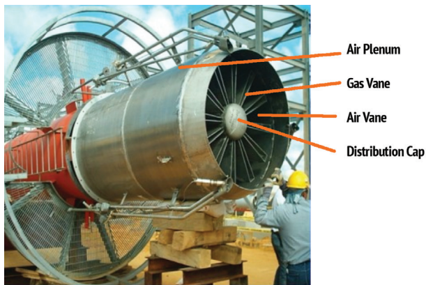
Figure 2. Integral components of an air flare tip.
