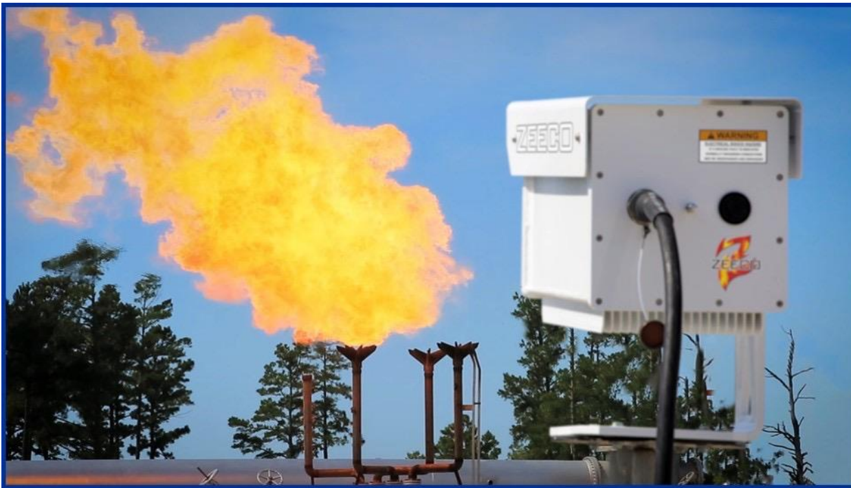
Figure 4 – Zeeco FlareGuardian monitoring system in use during validation testing
