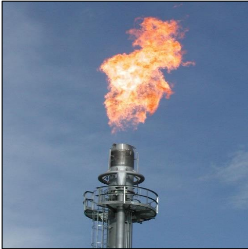
Figure 1 – Example of Air Assisted Flare
