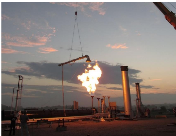
Figure 5 – Extractive Sampling Method Used for Testing
