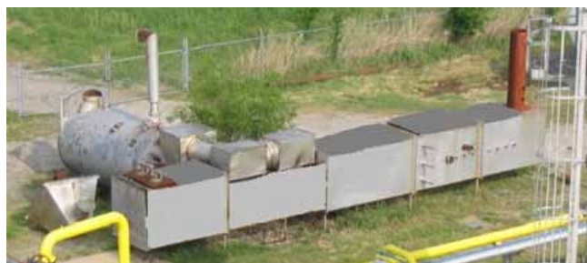
Zeeco's Duct Burner Test Rig. The simulated TEG is cooled by a running the TEG through a boiler to control the TEG inlet temperature to the duct runner at the correct temperature.
