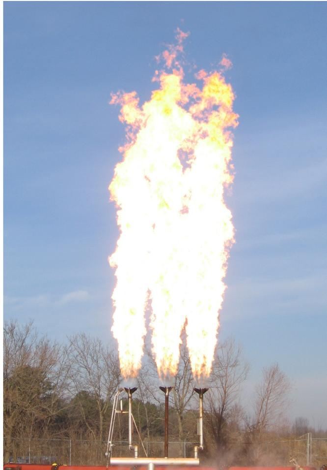
Figure 5 – Experimental measurements of flame shape, flame height, and radiation flux from a three-burner test firing ethylene under “no-wind” conditions.
