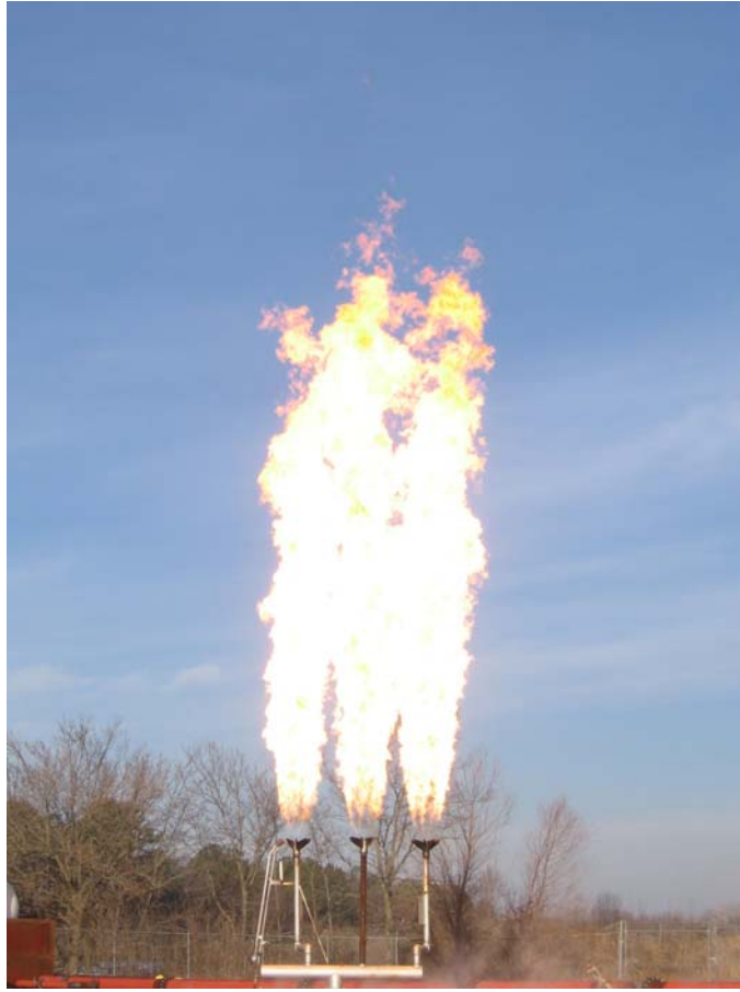
FIGURE 8: Multiple Burner Tip Testing
