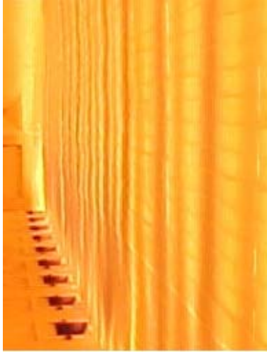
Figure 4: Zeeco’s GLSF Min-Emissions Flat Flame Burner. As shown on the left, the GLSF burner in operation with no flame rollover or flame interaction issues. As shown on the right, a diagram depicting the close proximity of the Zeeco’s GLSF burners in Wilson’s revamp application.
