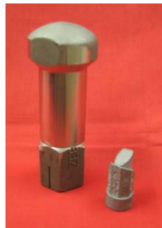
Figure 5. Zeeco’s airfoil tip design (shown right) has less mass and less exposed area, reducing temperature gain and coking.
