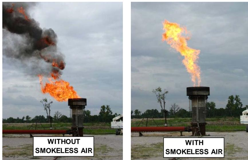
**Figure 10. Combustion Testing of HPAAS Flare at Zeeco**
