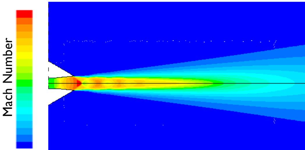
**Figure 8. Supersonic nozzle CFD velocity profile**
