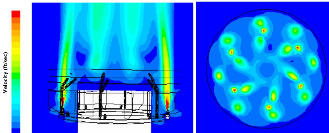
**Figure 9. HPAAS flare tip CFD velocity profile**
