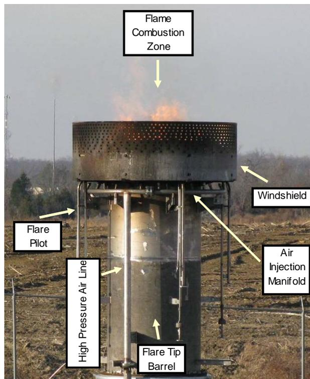
**Figure 6. Main components of HPAAS flare tip**
