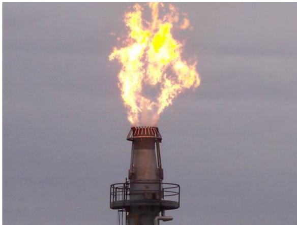
**Figure 3. Steam-assisted flare tip**
