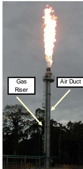
**Figure 5. Low-pressure air-assisted flares**
