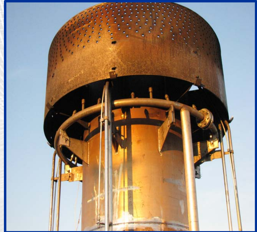
HPAAS tip can be operated for long periods of time with NO cooling air.
