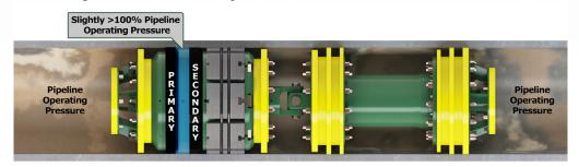
Both seals are proven in-situ to full pipeline pressure and the void between the seals is bled to ambient and locked-in for monitoring.
