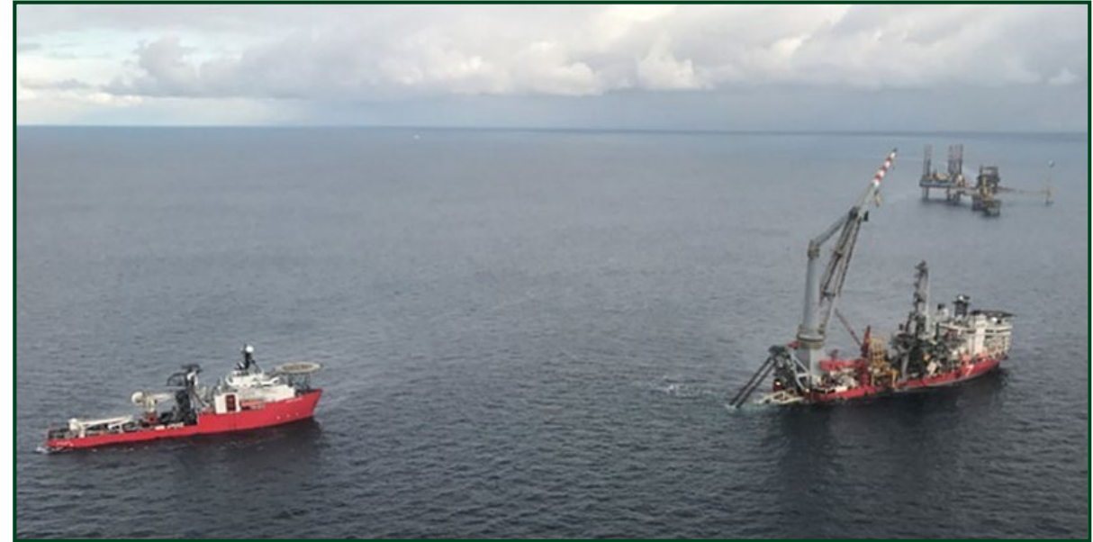
Pipelay of the new 26" bypass pipeline in early 2018. The pipeline will ensure export from Southern oil fields during shutdown
