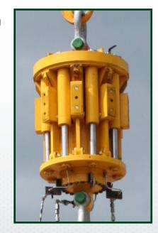
stabilisation within the caisson. The modular design of the ILT allows the length between lock modules to be configured to client requirements, this also allows for easy installation particularly in areas of restricted access.
