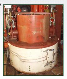
particularly in areas with restricted access or height. External gripping locks are hydraulically activated applying vertical load to the ELT which is set against the caisson.
