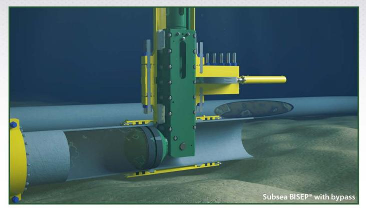
The BISEP when deployed subsea provides the highest level of hot tap installed pipeline isolation in the industry. Complying with all relevant subsea isolation guidelines, the BISEP ensures safe worksite conditions for divers from breaking containment to reinstatement.
