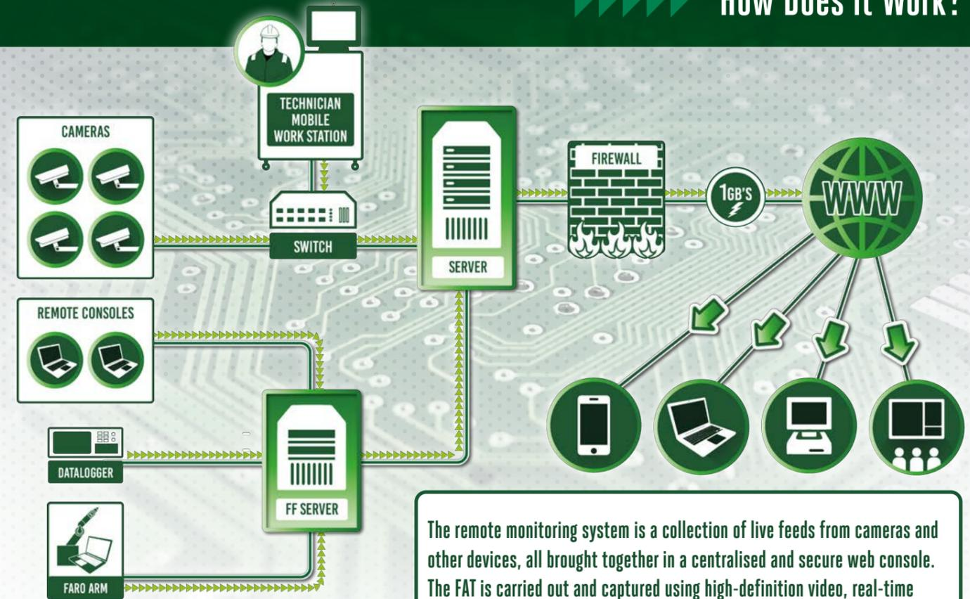
The remote monitoring system is a collection of live feeds from cameras and other devices, all brought together in a centralised and secure web console. The FAT is carried out and captured using high-definition video, real-time voice communication and file sharing to allow two-way communications and interaction between clients and our on-site team throughout testing.
